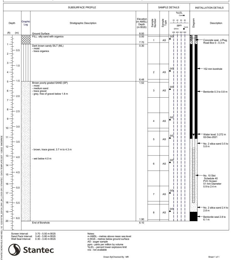
Screen Interval: Sand Pack Interval: 3.70 - 5.50 m BGS 3.40 - 5.80 m BGS
