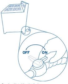
Turn valve so it is at a right angle to the pipe.
