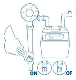
The gas supply shut-off valve is located where your gas service connects to your meter. To close, turn the valve a quarter turn with a 12" to 16" adjustable wrench or shut-off tool.
