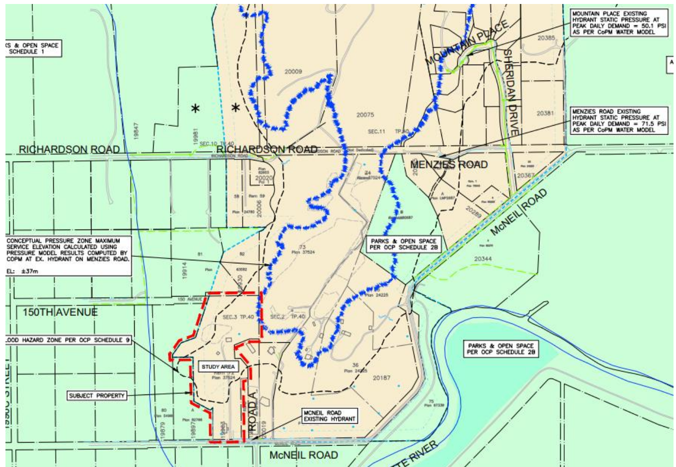
Figure 1: CoPM Water Model Simulation Hydrant Locations
