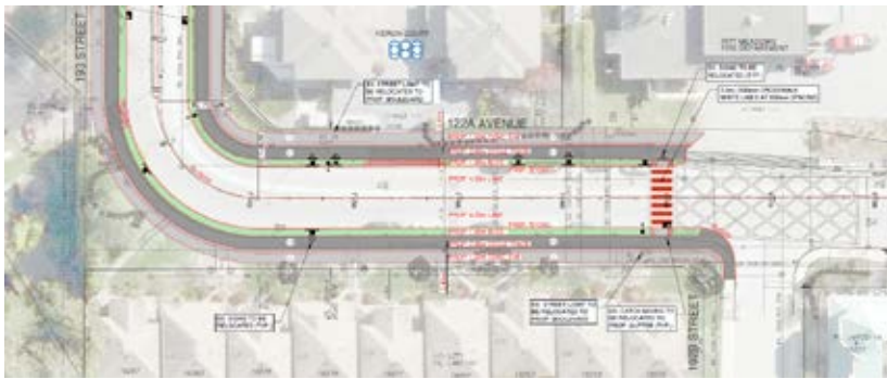
FIGURE 2 – MULTI-USE PATH AT 122A AVENUE
